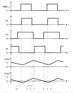
Fig.3. Timing sequences for CCM1 and CCM2 under SR.
