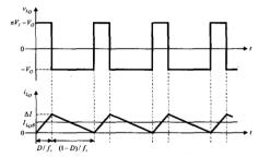
Fig. 2. Current flowing through  $L_{\rm O}$  on the boundary between CCM and DCM under no SR, along with the voltage across Lo.
