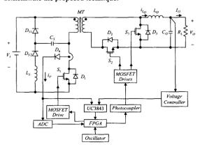
Fig. 1. System configuration of the experimental forward converter.
