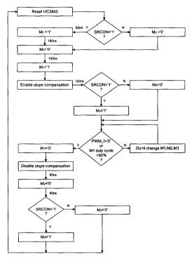
Fig. 7. How to generate the timing sequence for  $M_1$ ,  $M_2$  and  $M_3$  based on SRCON.
